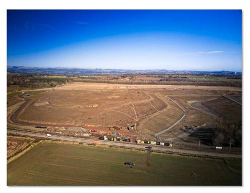
Remediation of the Auldcathie site was zoned based on the findings of earlier investigation, waste delineation during remediation and the proposed end use of the area. The core of the strategy was to provide an engineered landfill cap and gas collection system across the main biodegradable landfill with works area. comprising waste reprofiling and construction of a composite geosynthetic and geological
